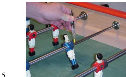
Apply 1 drop of lube to the inner rod We recommend Super Lube.
